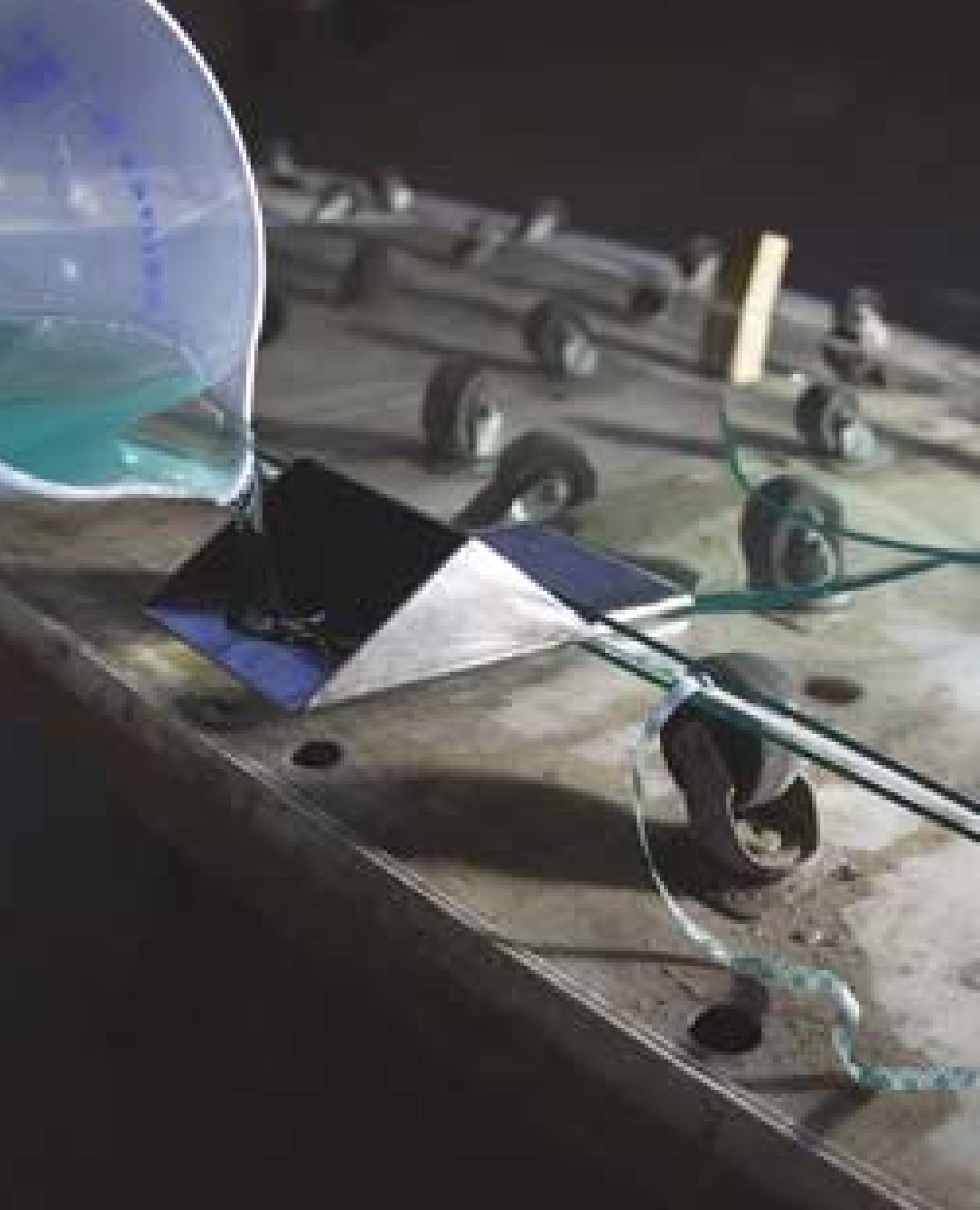
The Rankin Group are leaders in supplying specialist laminated glass from the delicate antique glasses to the heavy laminates for glass floors and large aquarium. The type of laminating used is 'cast in place' (CIP). Resin is poured between panes of glass and then cured.
